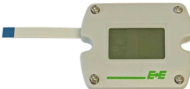
Fig. 7 FFC cable connection on the Sigma 05 electronics board
