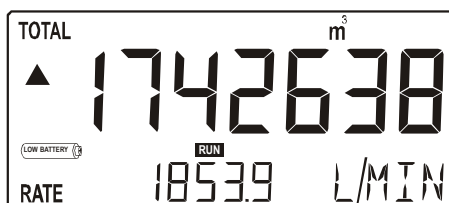
Fig. 4: Example of low-battery alarm.
