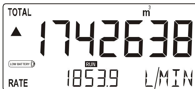
Fig. 4: Example of low-battery alarm.
