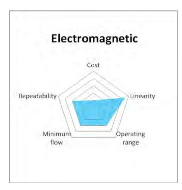
The fluid is the conductor and therefore the Electromagnetic meter is limited to fluids that can conduct electricity, however modern meters can measure flows in liquids with quite low conductivities.
