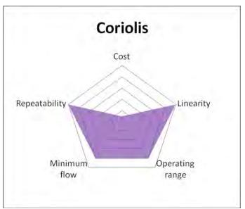
With the Coriolis, there is no obstruction in the bore (although the flow path can be very contorted) but these meters can be very accurate, with linearity's quoted down to  $\pm 0.1\%$ . Coriolis type meters are also usually very expensive.
