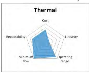
thermal element puts heat into the fluid and the dispersal of this energy is registered and converted into a flow reading.
