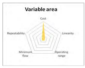
hospitals. This is a simple plastic or glass tube with a shaped float or ball that rises up a tube, whose cross sectional area changes up its length, hence the name variable area meter.
