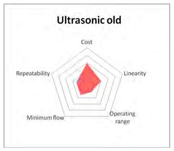
This makes these devices Reynolds numbers independent and can therefore operate from laminar flow right up to turbulent flow; in other terms, accurately measuring liquids ranging from water to high viscosity oils. Being through-flow devices they can also be tolerant to impurities in the system which would cause havoc to meters with moving parts.
