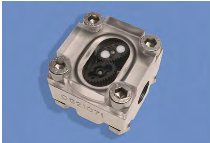
The basic oval gear flowmeter system is available with a transparent lid to allow visual observation of the rotating gears as an immediate flow indication. Bodies can be made from stainless steel, aluminium or PEEK. Electronic flow sensing uses Hall effect detection of the rotation of a ceramic magnet embedded in the rotor.
