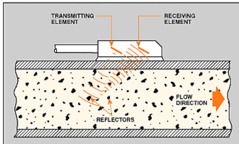
Katronic Flow meters can be configured to operate in Doppler - NoiseTrek™ mode. This mode is particularly suitable for fluids with a high solid or gaseous content and relies on solid particles or gas bubbles to give a flow rate reading.
