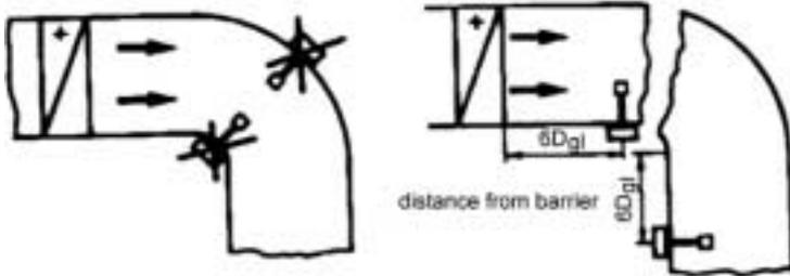
The following pictures are guidelines for correct installation of air velocity transmitters. Reliable measurements can be made by positioning the transmitter after filters (clean rooms), air heaters or air coolers, where the turbulence is very low.
