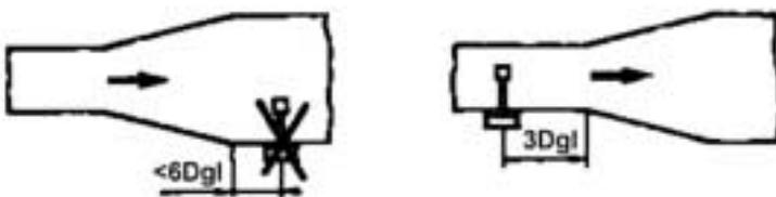
The probe shall be placed in front of diffusers or confusers.
