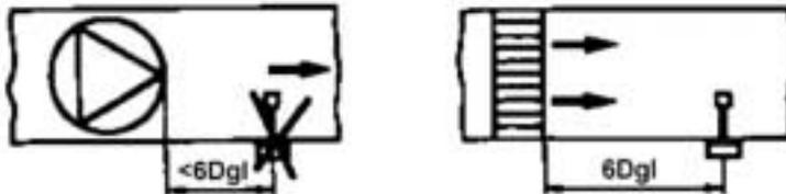
Preferred location after filters, rectifiers, coolers (no turbulences)
