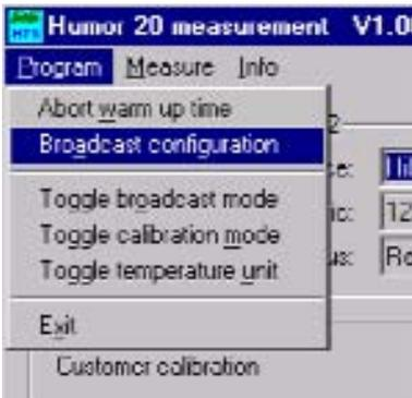
In Broadcast Mode the measured values from HUMOR 20 as well as all error messages are recorded continuously in a Log-file and displayed simultaneously on the monitor screen.
